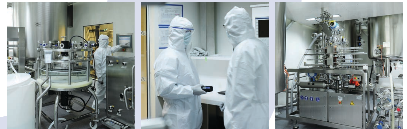
Ion exchange chromatography system, team working on the implementation of the new immunoglobulin product equipment and process and the new ultrafiltration system
