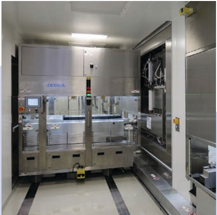
The new SVP filling line: vial washing machine, signal cables, automatic unloading cart for emptying the freeze dryers and 25m unloading corridor for emptying the freeze dryers
